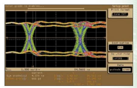
link between two nodes in such a way that a pseudo random binary sequence (PRBS) is transmitted. The result is a fully developed eye diagram. It is important to issue the packet from the Root Node, allowing it to transmit data with no request for the bus, thus making the data easier to trigger with less arbitration.
